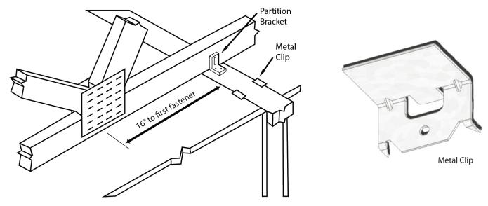
Where a narrow hallway is located at right angles to the roof trusses and drywall screws are held back 400mm from the wall on each side, there may be insufficient bottom chord length available to attach the drywall to the trusses. In this case, the best solution is to install separate 38x39 ceiling joists that are supported at each end by the partitions, fasten the drywall to these joists and avoid fastening the drywall to the truss bottom chords.
