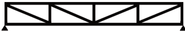
2X4 FLOOR OR ROOF TRUSS (CAN DESIGN WITH A CHASE AS WELL)
