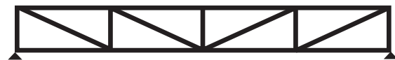
2x4 FLOOR OR ROOF TRUSS (CAN DESIGN WITH A CHASE AS WELL)
